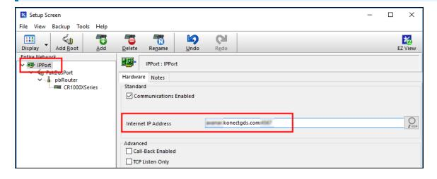
3. Leave the default settings for the PakBusPort. PakBus Port Always Open; it should not be checked. If you set an optional TCP Password, enter it on the PakBusPort Hardware tab.
