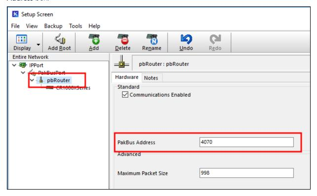
5. On the data logger Hardware tab, enter the PakBus Address chosen during the Set up Konect PakBus Router (p. 2) step.
