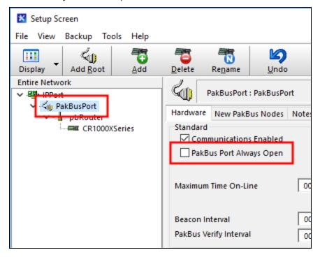
4. Select pbRouter from the Entire Network. On the Hardware tab, enter 4070 in the PakBus Address box.
